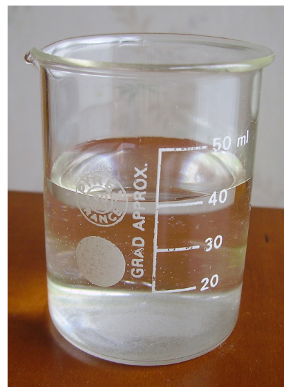
The volume of this water is approximately 40 ml. If you poured the water into a container with a different shape, its volume would still be the same.
